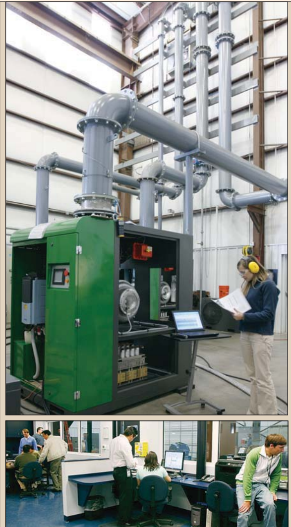
Shown above: State-of-the-Art blower test stand and customer viewing area
