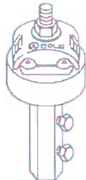
CC4B Conduit Cap to Cable Cast bronze cap with bolt pressure cable holder machined to fit snugly over 1-1/2" Schedule 40 PVC conduit. Has brass hex stock bolt pressure cable holder extending below. Stainless steel bolts, nuts and washer. Overall height 4.2" (10.6CM). Approximately 15.2 oz. (431 grams).
