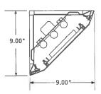
CC1 & CC2 – (4) .62" Mounting Holes CC4 – (6) .62" Mounting Holes 2
