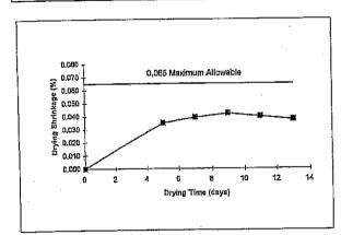
Comments: These units comply with the drying shrinkage requirements of ASTM C 90-09. Note: Final linear drying shrinkage, S, is calculated by averaging the final length measurement at equilibrium with the previous two measurements for each specimen.
